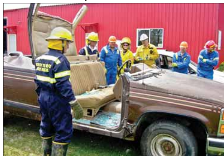
Vehicle extrication, training firefighters how to quickly dismantle a vehicle in order to remove anyone trapped inside.
